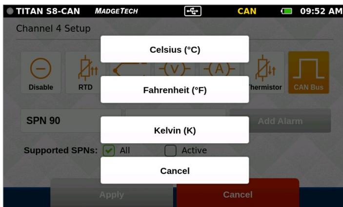
**Units:** These are the associated units for the specific SPN selected. For instance for engine temp = °F or °C. For fuel level = 0-100%, etc.
