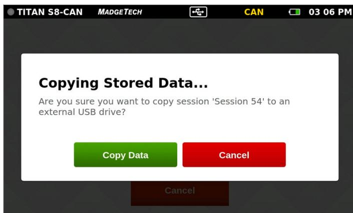
**Note:** Data can be saved to external memory as .csv and/or .mtb file format (user selectable in System/File Format).
